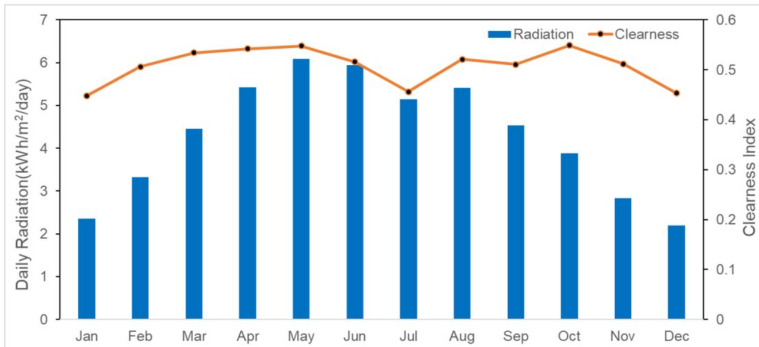
Figure 3: Solar source data at Gageodo Island
