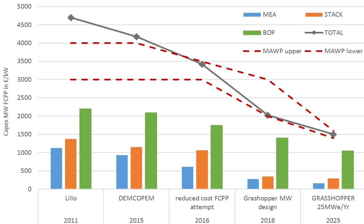
Figure 2 – Reduction of CAPEX in the multi-MW FCPP.
