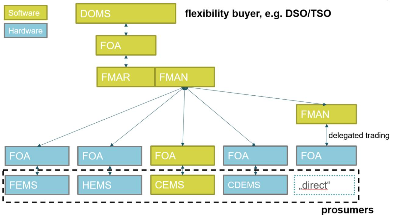
Fig.1: Architecture of the GOFLEX flexibility trading system [4].
